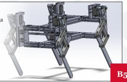
The challenge of our project is to design a solar powered terrain walker. The walker uses a chebyshev mechanism to produce forward motion. The walker is charged by a solar panel attached at the top.
