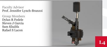
Developing a novel 3D printer head capable of storing plastic pellets and extruding them at high temperatures for improved materials science research.
