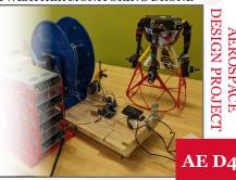
This project is a tether system that continuously powers a weather monitoring drone at altitudes up to 200 feet. It consists of a cable and an automated reel that manages tension in the tether wire.
