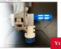
We designed a pneumatic soft gripper to be attached to a robotic arm for fast manipulation of parts from a bin to a fixture.
