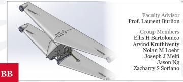
The exoskeleton aims to transport a human while being similarly sized. This project is a scaled down version using electricity to power its flight. It will transition from vertical takeoff to horizontal flight and back
