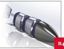
A mechanical fish prototype that can swim in a straight line automatically using Arduino code and make turns using undulatory motions, with battery power.
