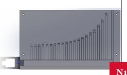
This project is an educational working hydrodynamic model of mechanical sound wave filtering in the human cochlea. It demonstrates Békésy's classical passive wave theory, which is fundamental to understanding cochlear mechanics.
