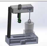
Developing a device utilizing torque, texture analyzing, and optical analysis to assess mixedness of dense pastes, targeting manufacturing efficiency and accuracy.
