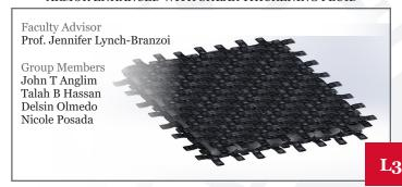
An experimental liquid armor developed involving a combination of features from previous designs in order to reduce the impact felt by blunt trauma while keeping armor thickness low.
