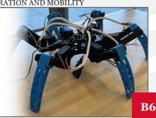
This project aims to develop a solar-powered walking vehicle meeting specifications like a 1.5-foot height limit, autonomous obstacle avoidance, and an 8-ounce payload. It will race a rival team, utilizing solar energy stored onboard.
