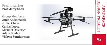
An autonomous drone equipped with advanced sensors and control systems to map wind flow velocity in Rutgers' Windshaper wind wall, providing accurate data for aerodynamic research and simulation validation.
