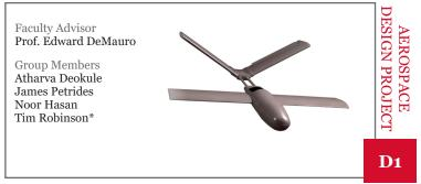
This project is a deployable glider capable of autonomous, targeted guidance during flight. Its objective is to complete mission 3 at the American Institute of Aeronautics and Astronautics (AIAA) Design, Build, Fly (DBF) competition.
