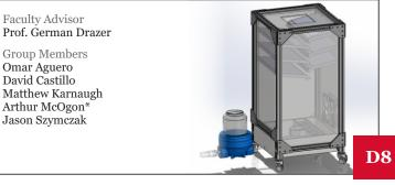
A compact, liquid-based air filtration system that uses water to capture and remove airborne pollutants, improving air quality. Designed for portability, it offers an innovative solution for cleaner and healthier air in any environment.
