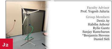
A wind driven water system that stores and pump water for agriculture irrigation system implementing wind turbine, centrifugal pump, Arduino controlled valves, and automated water supply system.
