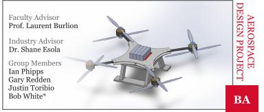
This project aims to create a durable, lightweight, and thrust efficient drone that can carry a payload that is heavier than itself. The quadcopter design features four folding arms with each having two coaxial rotors.
