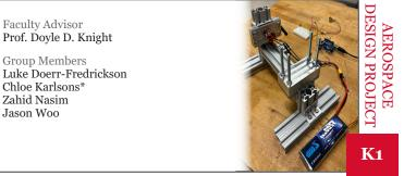
A motor generator test stand utilizing brushless DC motors and an Electronic Speed Controller to analyze power transfer, torque, efficiency, and performance characteristics in an experimental setup.
