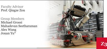
Designing, modeling, building, and operation of an autonomous robot that can manipulate rings, move mobile goalposts, and climb rungs to score points in the VEXU High Stakes Skills Challenge.
