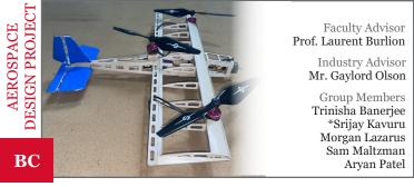
Develop a non-conventional drone that seamlessly transitions between helicopter and fixed wing mode to maximize efficiency and negate the need for a runway.
