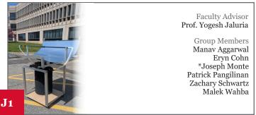
A small-scale solar collector designed to heat household water efficiently. It captures sunlight, converts it to thermal energy, and warms water for daily use, offering an eco-friendly, cost-effective solution for domestic hot water needs.
