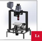
A cost-effective thermoplastic pellet-fed 3D printer featuring a moving heated bed and stationary extruder, designed for enhanced scalability, material diversity, and sustainability in additive manufacturing.
