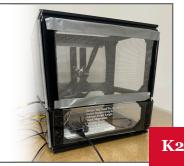
A test stand for RC electric motors measuring torque, power, current, and RPM. It includes an IR sensor, Arduino-based data collection, a power sensor, adjustable motor and IR sensor mounts, and an aluminum frame, ensuring accurate, repeatable performance evaluation within budget constraints.
