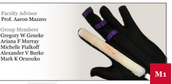
Our project utilizes a hybrid design of a cable system, as well as pneumatically actuated inflatable bladders to assist in the opening and closing of a users hand. This process aids in the repetitive motion physical therapy exercises used to strengthen the grasp of people with sustained issues of motor control such as stroke patients.
