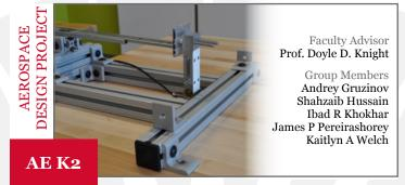
A stand capable of measuring 5-50 N of thrust from various model rocket engines with an accuracy of  $\pm 5\%$ . The data is wirelessly transmitted to the computer interface where it can be graphed and analyzed.
