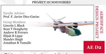
This long range search and rescue platform has combined the hovering capabilities of a quadcopter with the high efficiency of an airplane to acheive a powerful combination boasting the fastest transition time in the industry.
