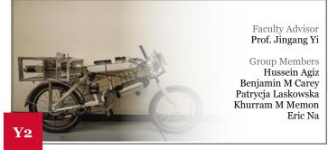
Self-stabilizing single-track bicycle capable of maneuvering through narrow spaces and carrying payload. Ideal for situations where a bulky machine, drone, or person would not be efficient.
