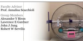
Our project is a spherical robot that is capable of quickly rolling, stopping, and changing direction. Our ideal environment is a relatively smooth surface at a maximum incline/decline of 5 degrees relative to balance.
