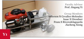
Autonomous Grinder that implements dry grinding by using a single grinding disc to grind and polish concrete floors. A vacuum is attached to the grinder to retrieve all the dust produced by the grinder.
