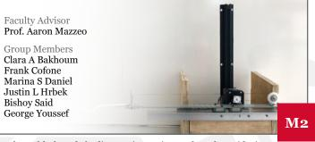
The cable-based feeding assistant is a robot that aids in feeding those who do not have full use of their arms. It is made up of two arms and a wrist joint that are run by a cable-based pulley system powered by stepper motors. The purpose of building a robot that is cable-based is to improve safety, control over the movements, and decrease the inertia by limiting movements.
