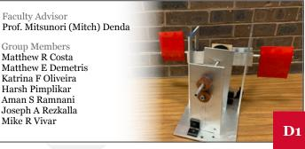
Climate change is a priority issue. Unlike windmills or solar farms, this bio-inspired flapping wing energy harvester is a machine designed to harvest wind energy for lower wind speeds. This model can be scaled up to provide energy for residential/commercial applications in order to reduce fossil fuel consumption.
