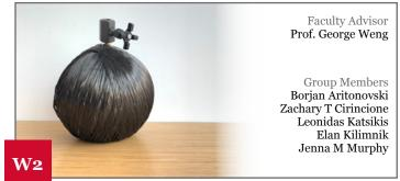
A lightweight, high-strength, composite overwrapped spherical pressure vessel made from a carbon fiber and epoxy matrix shell and a rubber interior bladder that is useful in aerospace applications.
