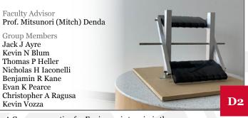
A Common practice for Engineers is to mimic the complexities of nature itself. This is highlighted in the BESTO, a bio-inspired flapping wing wind energy harvester. While typically unwanted in aspects of aeronautics, wing tip vortices can be utilized immensely for the purpose of energy harvesting. The BESTO uses these recent discoveries to increase efficiency and ultimately gain a leg up on other common wind-energy hardware.
