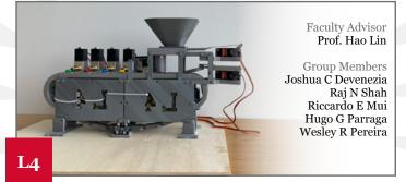
A conveyor belt based system which receives items with close geometric homogeneity and distinguishes them non invasively by topical finish using a sensor. The characterized items are carried by the conveyor belt to be separated into bins by pneumatic actuators responding to an Arduino signal.
