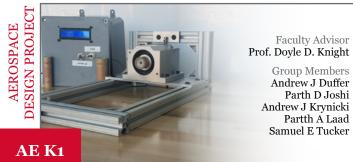
The Rocket Engine Thrust Stand accurately and safely measures the thrust of model rocket engines. It will be used as a laboratory experiment to provide future engineering students hands on experience with rocket propulsion.
