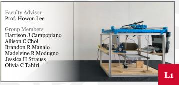
This 3D printer produces an object through selective deposition lamination using recycled paper as the medium. Each layer of paper is applied glue, heated and compressed, and then cut into the desired shape.
