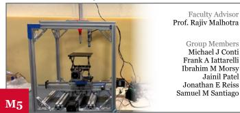
Inspired by challenges in the construction of sustainable shelters in disaster stricken areas, the innovative 3D Dust Printer was developed to provide a way to construct structurally stable construction materials with limited resources. The printer operates by extruding a mix of local particulate materials and a resin, while simultaneously passing a UV light overhead to cure each layer.
