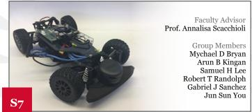
This project designs and programs an RC rover to navigate an obstacle course autonomously. The car uses data inputted from a LIDAR sensor and is built to compete in the annual F1Tenth Autonomous Racing Competition.
