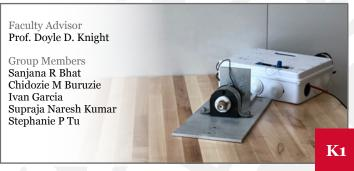
Our group is designing and fabricating a model rocket thrust stand, that utilizes a button load cell. The load cell captures thrust in the x-axis. This data is then transferred to an Arduino that can wirelessly send it to the computer. While capturing data, it is presented on a LabView interface. The data can be saved from LabView and sent to anyone. Additionally, our model rocket thrust stand is highly manufacturable, thus making it simple yet effective.
