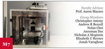
Our goal is to create a 3-D printer that prints using a two part epoxy mixture. Our epoxy printer will be embedded with continuous fibers, providing objects with stronger mechanical properties and high temperature resistance.
