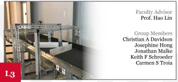
Our conveyor belt sorting mechanism will contribute to creating a more efficient way of recycling metal scraps. The design utilizes chicaning in the organizing process and color detecting sensors in the sorting process.
