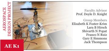
Tabletop test stand to download real time thrust (in the range of 5 to 20 Nt), input electric power, and rpm data of an RC motor and propeller.
