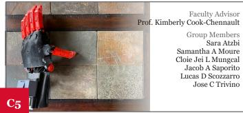
A 3D-printed prosthetic hand based on the e-NABLE Phoenix Hand v2 model which has been modified to house a mechanism that allows the user to draw/release a bow & arrow.
