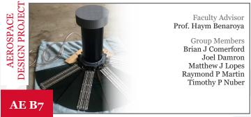
A Hybrid Lunar Inflatable habitat designed to function as an early Lunar base in a series of Moon missions to develop a Lunar colony. The model built demonstrates the deployment of the structure, including inflation.
