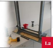
Three step design to create commercial grade 3D filament to be input to a 3D printer for demonstration, including shredder and heating chamber.
