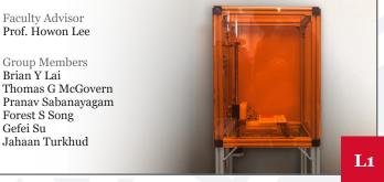
Using digital light projection, our printer is capable of 3D printing ceramic parts with higher density than current commercial options, resulting in parts with less shrinkage and porosity post-sintering.
