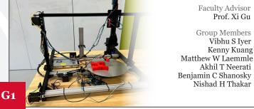
A modified gantry capable of performing different functions related to the manufacturing of items. The gantry autonomously switches functions to manufacture products without human intervention once commands have been sent in.
