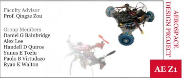
An autonomous drone provides a "map" of an area for the ground rovers to follow and bring the package to its destination.
