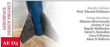
RRPL's two-stage rocket has struggled with static stability due to opposing forces, and with drag at supersonic speeds. Through research, we created a custom airfoil and fin shapes to optimize stability without compromising drag.
