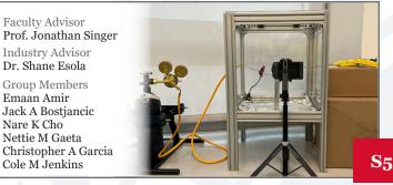
The MINET materials manufactured in Dr. Singer's Laboratory present interesting potential for extracting and moving high amounts of energy. With our partners at Picatinny Arsenal, we built a combustion chamber to safely observe their properties.
