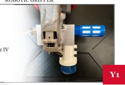
We designed a pneumatic soft gripper to be attached to a robotic arm for fast manipulation of parts from a bin to a fixture.
