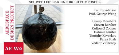
A lightweight spherical pressure vessel made from carbon fiberreinforced polymer composites. Our design utilizes a geodesic sphere as the internal structure with an interior rubber bladder. Cover Photos (All group members listed left to right):
