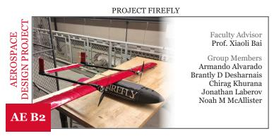
A long range, unmanned aerial vehicle designed for inflight aerosol measurements and sampling for wildfire monitoring. Capable of autonomous, real-time aerosol monitoring for fire evacuation, flame front monitoring, and air sample collection for further analysis.
