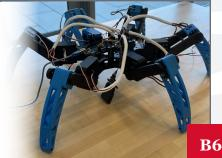
This project aims to develop a solar-powered walking vehicle meeting specifications like a 1.5-foot height limit, autonomous obstacle avoidance, and an 8-ounce payload. It will race a rival team, utilizing solar energy stored onboard.
