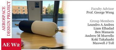
Type 4 Carbon fiber cylindrical pressure vessel which is about 3.5 times lighter than that metallic tanks. Manufacture through the wet winding process prioritizing minimal thickness of carbon fiber layering.
