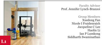
The project goal is to modify a standard FDM 3D printer to be able to print elastomeric composites. This is accomplished by implementing a pump system that will transport the liquid elastomer material.
