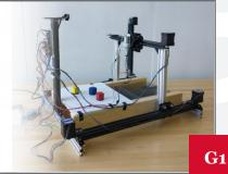
A three axis automated gantry system used to sort items via color into similarly colored receptacles. A camera is used for object detection and the system will run autonomously.
