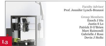
Building a custom extruder on a Lulzbot Mini capable of printing from thermoplastic pellets rather than filament. Allows for researchers to more easily test novel materials using the flexibility of 3D printing.
