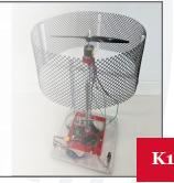
Tabletop Electric Engine Thrust Stand capable of measuring thrust, voltage, current and revolutions per minute of a motor and drone propeller.
