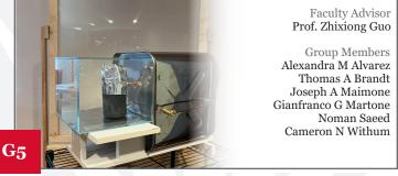
The Solar-Powered Water Purifier is a device which utilizes a fresnel lens to harness solar energy and in turn powers a water purification process that boils contaminated water to generate and condense purified steam.
