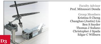
This is a device that generates electrical energy using a mechanism based on the flapping motion of bird wings. Incoming wind causes the wings to flap, which are then connected to a generator.
