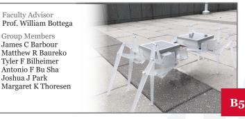
This project features a solar powered terrain walker, featuring independently controlled Klann linkage mechanisms as legs, a hinged body design for flexibility, and can navigate over or around uneven terrain.
