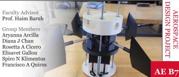
A reaction control system and avionic system for rockets that will adjust fin rotation to reduce the effect of pitch and yaw moments to maximize apogee.
