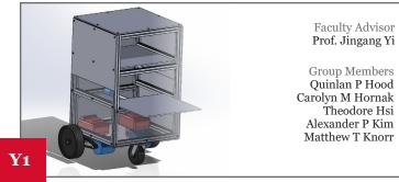
An autonomously navigating delivery customer service robot intended for settings such as a hospital or a restaurant to ease the workload of employees.
