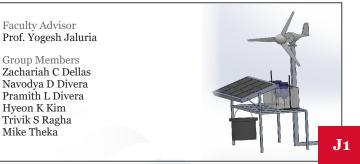
Hybrid wind turbine and photovoltaic panel for energy harvesting plus electrolysis tank for hydrogen collection, integrated with electronics for system operation and data collection.
