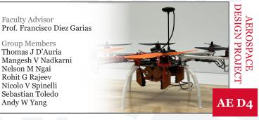
A hexacopter has a mechanical claw system with the purpose of picking up and delivering medical supplies. The drone features a servo motor-driven 3D printed mechanical claw to clamp down on supply packages.
