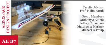
This project determines the stability and control characteristics of an aircraft using on-board motion sensors to create mathematical models. Thus, the resulting motion will be related to the corresponding deflection of control surfaces.
