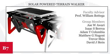
Custom-built, remote-controlled, table-top sized terrain walker fully powered by solar panels, designed to quickly navigate various terrain without wheels while carrying a small payload.
