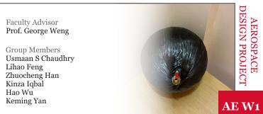
A spherical pressure vessel was constructed using carbon fiber filaments and epoxy resin. The epoxy resin is applied to a spherical mold and carbon fiber filaments are wound around the sphere and cured with air.
