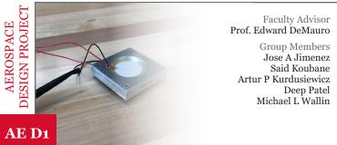
A synthetic jet actuator is a device that can be used to enhance the performance of an airfoil at high angles of attack when flow separation is a concern.
