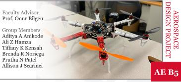
The goal of this project is the design, analysis, fabrication and testing of a small quad-copter unmanned aerial vehicle (UAV) to act as a platform to conduct Zero-G experiments
