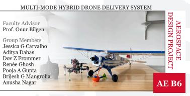
An autonomous multi-UAV delivery system using a fixed-wing airplane carrying a quadcopter over long distances. On arrival the quadcopter undocks, drops off the payload, and re-docks, allowing the system to continue its journey without landing.
