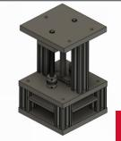
The non-destructive material identification device will be able to electronically determine the type of material using the displacement under a given load.
