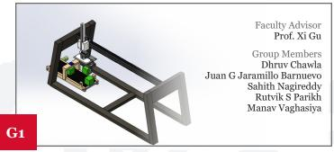
Tabletop automated gantry system using Arduino sensors and motors to move fragile objects within an assembly line in a XZ coordinate system.
