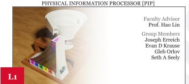
The physical information processor modularly sorts a random mass of objects by color. Objects are linearized into a single stream using a vibratory bowl feeder and then color-sorted using a sensor to activate motorized gates.
