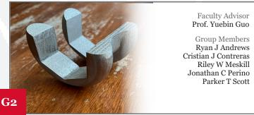
The original design, manufacturing, and analysis of a customizable knee implant. This project uses 3-dimensional design software, 3-dimensional printing in metal and polymer materials, machining of parts, and analysis software for product stress testing.
