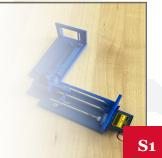
This device stretches skin and measures its displacement and the force applied to aid in the rearch of transdermal drug delivery.
