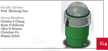
This device is designed to evaporate the salt water using the sunlight that will be concentrated on an aluminum heat chamber in order to yield clean, drinkable water.
